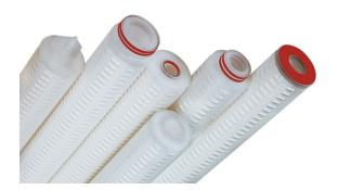
Additionally, the product water must be polished or filtered with a membrane, to reach the required cleanliness. In general, the polishing filter will utilize a 0.2µm hydrophilic membrane, with or without some form of bacterial retention. Appropriate regulatory agencies or in-house company guidelines will typically provide membrane requirements for your process.
